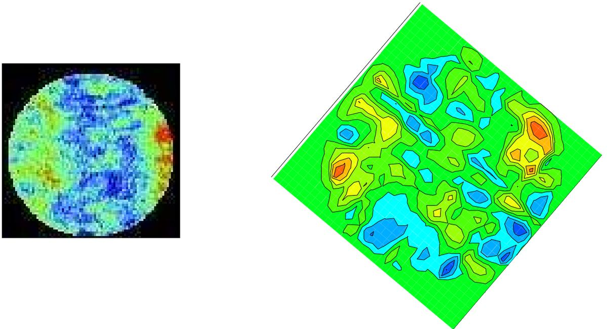
The enlarged wavefront from Veeco (on left) and the wavefront as measured by Sensoft (right). A clear correspondence between the two is seen. Some of them have been indicated above
